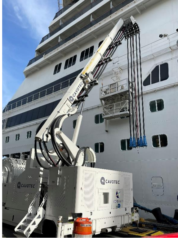
Figure 14- CMS unit in position, Matt Creswell
