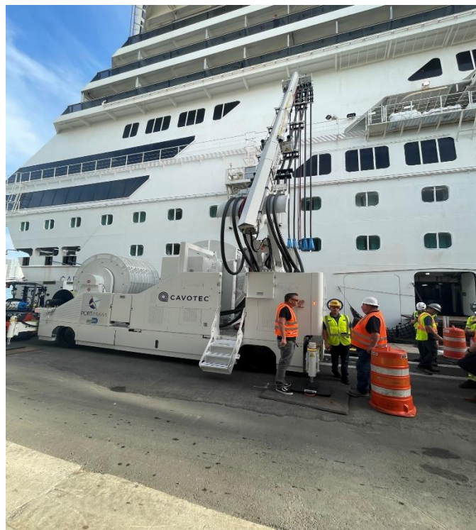
Figure 12- Cavotec CMS (cable management system) Unit, Matt Creswell
