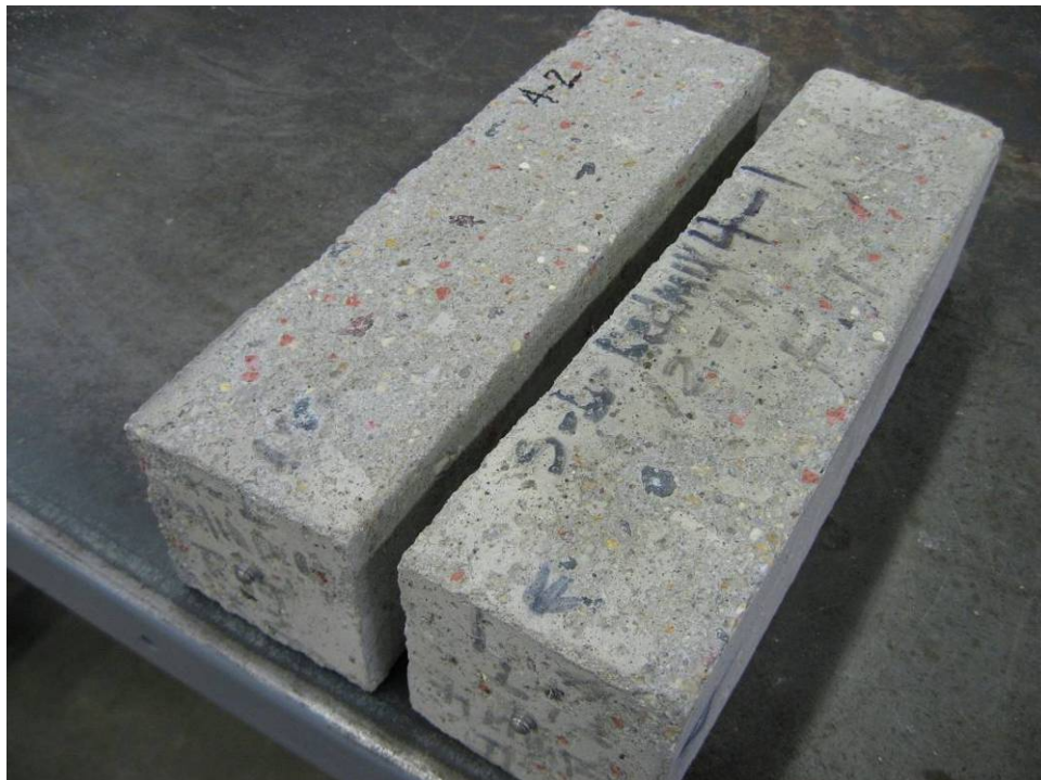
Figure 7. 3000 psi CCA at 100% Coarse Mixture After 300 Freeze-thaw Cycles
