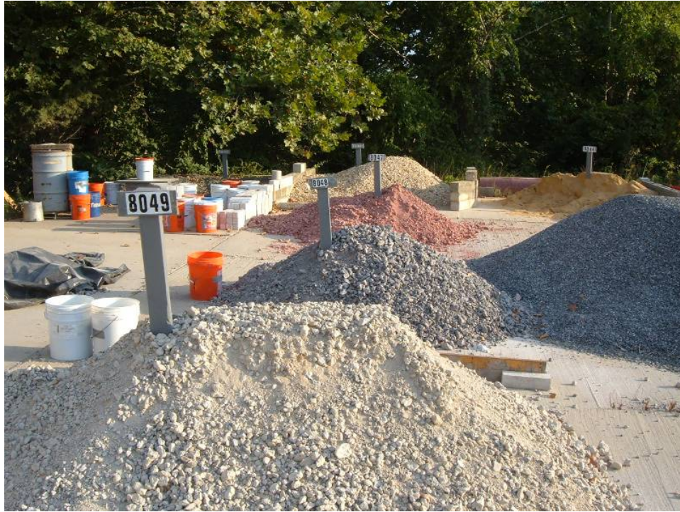
Figure 2. CCA Stored at NRMCA Research Laboratory (Red=3000 psi, Black=5000 psi, Gray=1000 psi)
